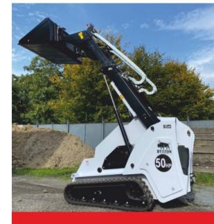
A tracked mini loader for work activities where high performance is required. The ultimate compact machine with comfortable joystick control equipped with a **telescopic boom** that enables unloading up to a height of over 3m!
